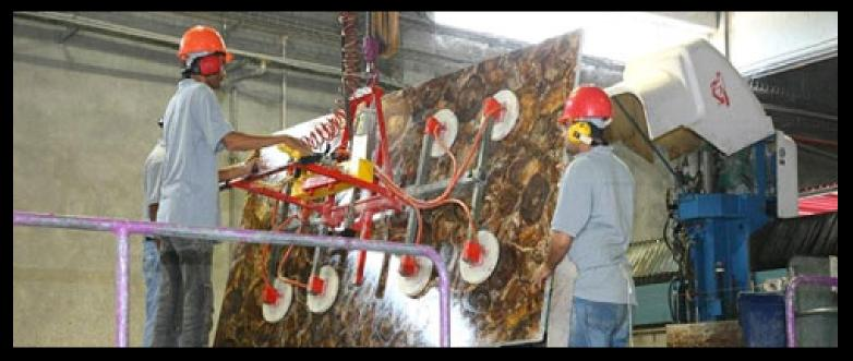
Once this painstaking work in arranging and filling is complete, the slab undergoes quality control processes that ensure homogeneity, mineral grade and slab design. The slab is then taken to the firing, calibration and cutting area where the final slab dimensions are obtained.
