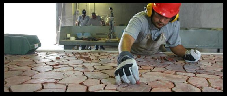
The next step involves the arrangement of the pieces. This process is completely handcrafted; that is, the pieces are arranged manually. The idea is to maximise the space and to create only the smallest of gaps between stones which will later be filled by resin and fused together. Expert artisans fill in the remaining spaces with semi-precious stones of smaller sizes in order to ensure that the resulting gap is as small as possible.
